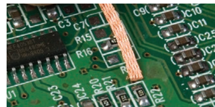
Match braid width to contact area
